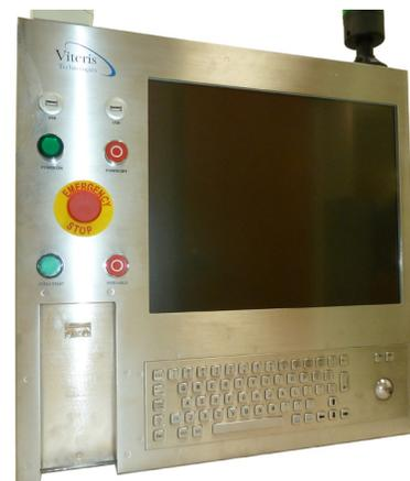
The control module is housed in a stainless steel enclosure that is mounted on a swing arm. It features a 19" touchscreen, full keyboard, trackball, and dedicated buttons for critical machine functions. A removable CNC pendant (not shown) is housed in the lower left recess.
